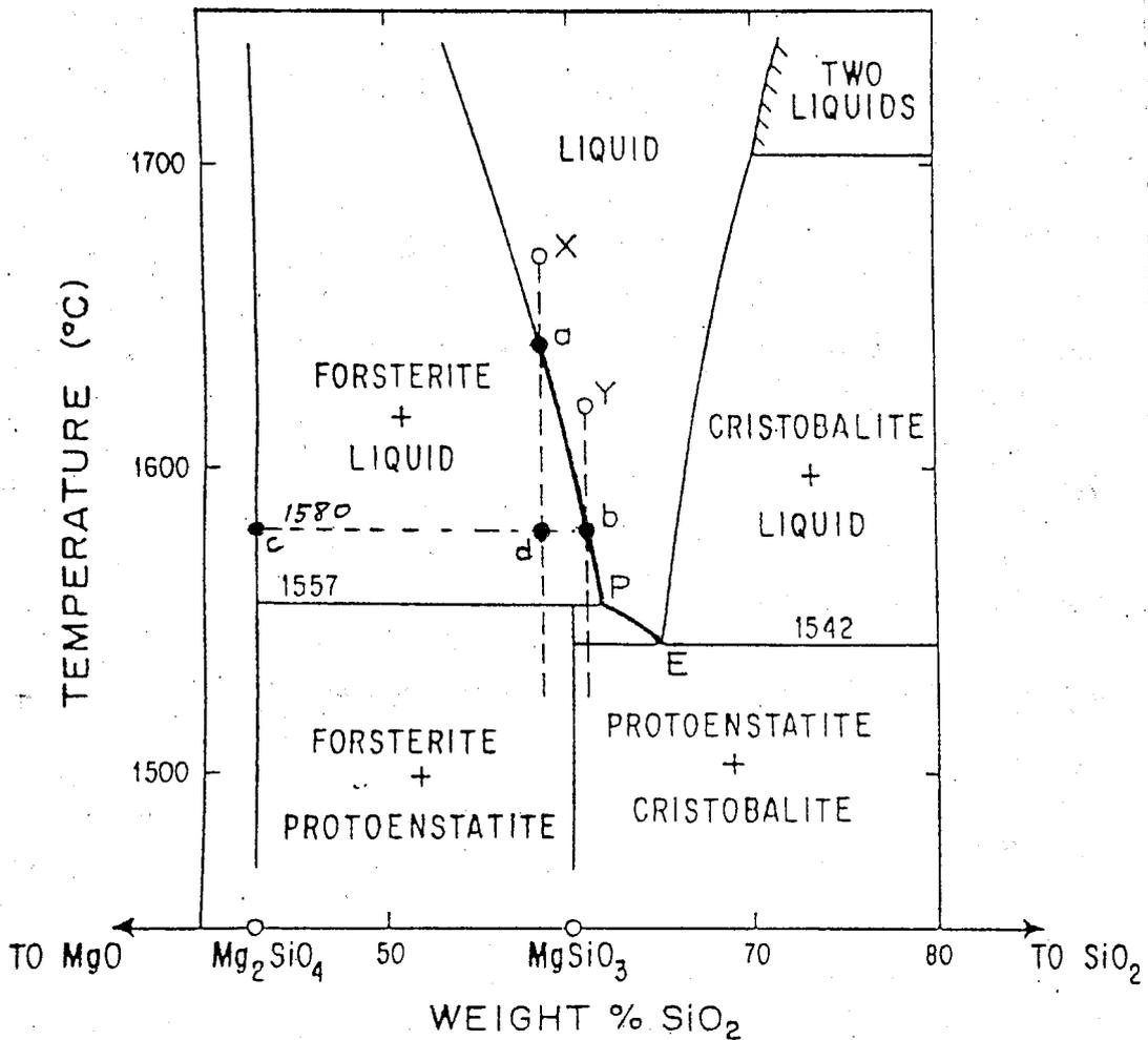
Figure Phase relations in the system MgO-SiO<sub>2</sub> (Bowen and Andersen, 1914), illustrating paths of crystallization for selected mixtures in the vicinity of the metasilicate (MgSiO<sub>3</sub>) composition.
